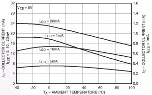
Fig. 16 - Current Transfer Ratio vs. LED Current
