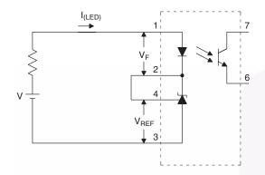
Figure 1. V<sub>REF</sub>, V<sub>F</sub>, I<sub>LED</sub> (min.) Test Circuit
