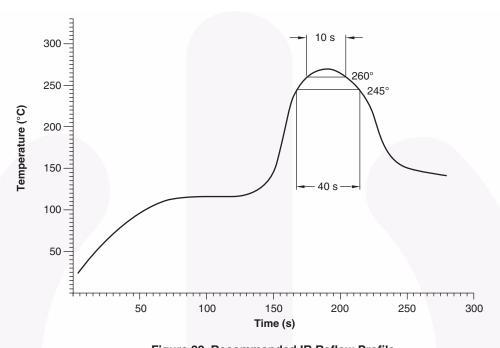
Figure 22. Recommended IR Reflow Profile
