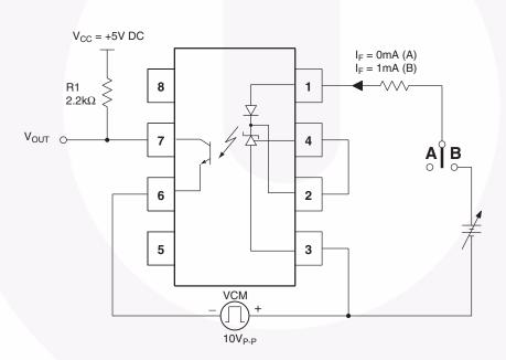
Figure 8. CMH and CML Test Circuit
