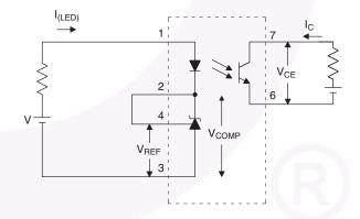
Figure 6. CTR, V<sub>CE(sat)</sub> Test Circuit
