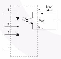
Figure 5. I<sub>CEO</sub> Test Circuit
