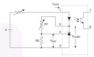
Figure 2.  $\Delta V_{REF}/\Delta V_{COMP}$  Test Circuit
