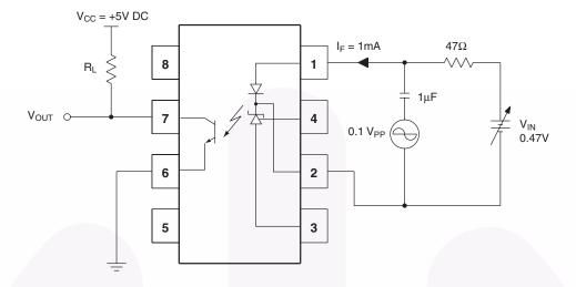
Figure 7. Frequency Response Test Circuit.
