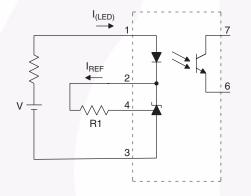
Figure 3. I<sub>REF</sub> Test Circuit
