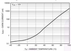
Fig. 15 – Collector Current vs. Ambient Temperature
