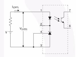
Figure 4. I<sub>(OFF)</sub> Test Circuit
