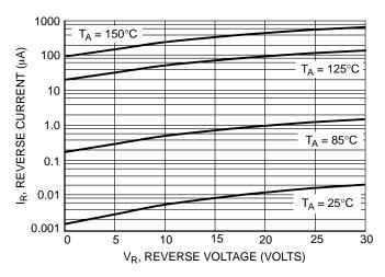
Figure 3. Leakage Current
