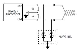
Figure 7. FlexRay Surge Protection Circuit
