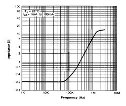
Figure 8. Dynamic Impedance Frequency
