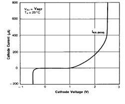
Figure 6. Cathode Current vs. Cathode Voltage
