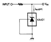
Figure 4. Test Circuit for I<sub>KA(OFF)</sub>
