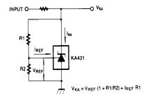
Figure 3. Test Circuit for  $V_{KA} \ge V_{REF}$
