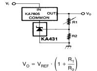
Figure 13. Output Control for Three-Terminal Fixed Regulator
