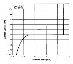
Figure 5. Cathode Current vs. Cathode Voltage
