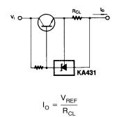
Figure 15. Current Limit or Current Source
