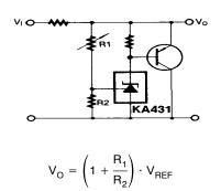
Figure 14. High-Current Shunt Regulator
