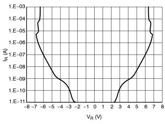
Figure 7. Breakdown Voltage
