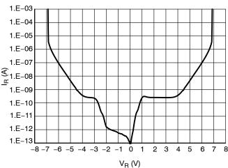
Figure 8. Reverse Leakage Current
