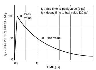
Figure 11. 8 X 20 μs Pulse Waveform
