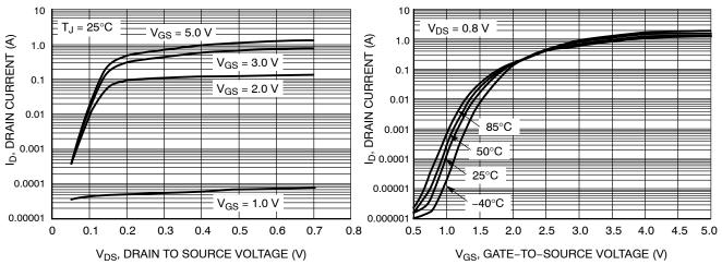
Figure 2. Output Characteristics
