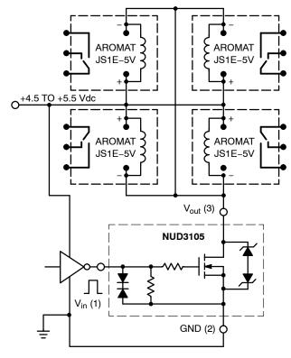
Figure 14. A Quad 5.0 V, 360 mW Coil Relay Bank
