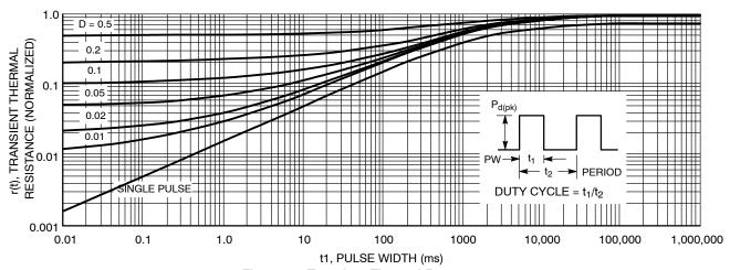
Figure 11. Transient Thermal Response
