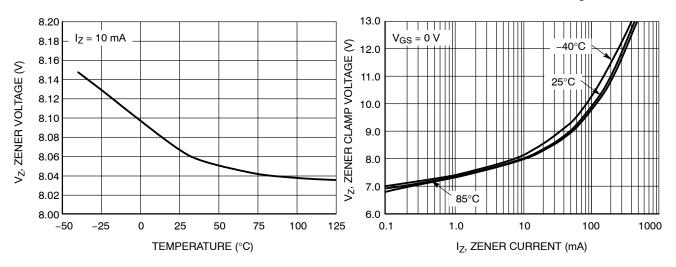
Figure 6. Zener Voltage vs. Temperature
