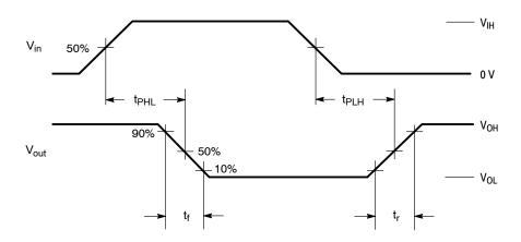
Figure 1. Switching Waveforms
