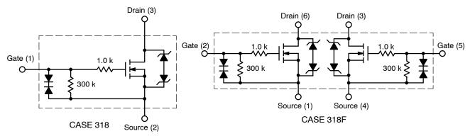
Figure 1. Internal Circuit Diagrams
