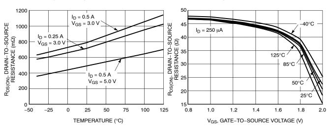
Figure 4. On Resistance Variation vs. Temperature
