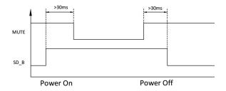
Figure 2. Recommended Power On/Off Sequence
