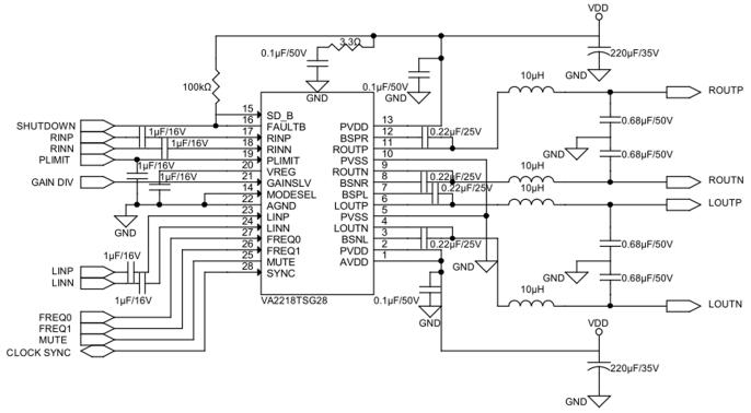
Figure 16. VA2218 TSSOP28 Stereo Reference Application
