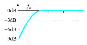
Figure 1. Cut-off point of high-pass filter
