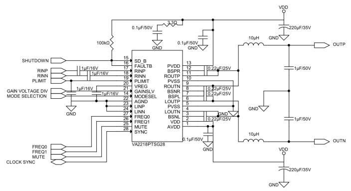
Figure 17. VA2218P TSSOP28 Mono Reference Application
