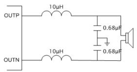
Figure 3. Typical LC Output Filter, Speaker Impedance= $8\Omega$
