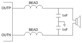
Figure 4. Typical Ferrite Chip Bead Output Filter
