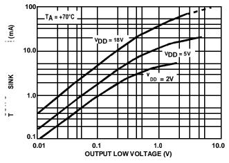
FIGURE 12. OUTPUT SINK CURRENT vs OUTPUT VOLTAGE
