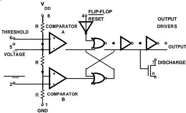
NOTE: This functional diagram reduces the circuitry down to its simplest equivalent components. Tie down unused inputs.
