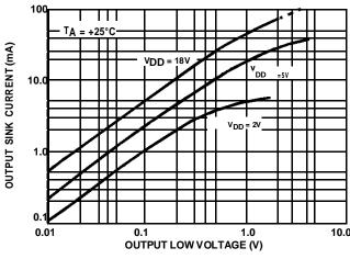
FIGURE 11. OUTPUT SINK CURRENT vs OUTPUT VOLTAGE
