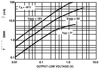
FIGURE 10. OUTPUT SINK CURRENT vs OUTPUT VOLTAGE
