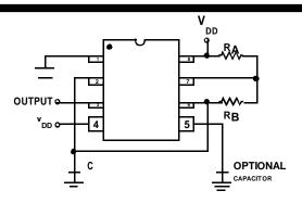
FIGURE 5. ALTERNATE ASTABLE CONFIGURATION
