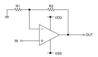
Figure 13. Non-inverting amplifier circuit
