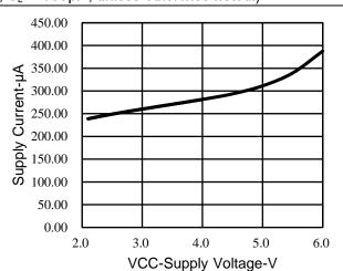
Figure 3. Supply Current vs Supply Voltage
