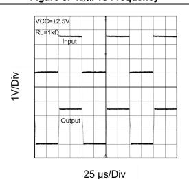
Figure 7. Noninverting Large-Signal Pulse Response
