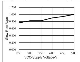
Figure 2. Slew Rate vs Supply Voltage
