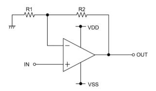
Figure 14. Non-inverting amplifier circuit
