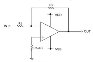
Figure 13. Inverting amplifier circuit
