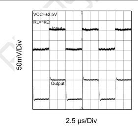
Figure 6. Noninverting Small-Signal Pulse Response
