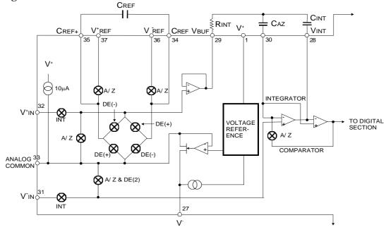
Above is the block diagram of the Analog Section for HT7106A.
