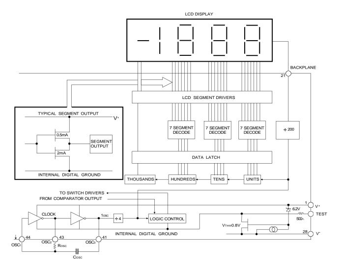
The internal digital ground is generated from a 6.2 volt Zener diode and a large pchannel follower. This supply is made stiff to adsorb the relatively large capacitive current when the back plane (BP) is switched. The BP frequency is the clock frequency divided by 800. The segments are driven at the same frequency and amplitude and are in phase with BP when OFF, but out of phase when ON. In all cases, negligible DC voltage exists across the segments.
