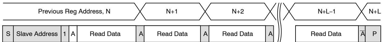
Figure 42. Sequential READ, Start from Current Location
