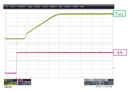
Figure 3. Typical Start–up with V $_{\rm IN}$  = 12 V, R $_{\rm OUT}$  = 6  $\Omega$
