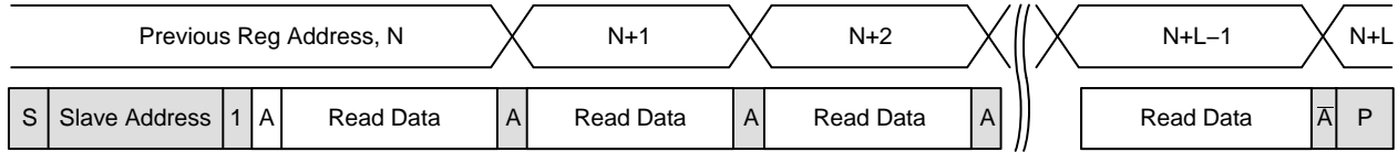
Figure 13. Sequential READ, Start from Current Location
