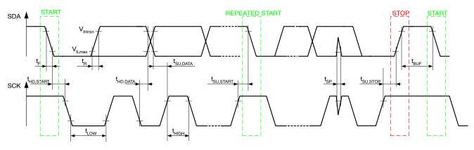
Figure 5. I<sup>2</sup>C Timing Diagrams
