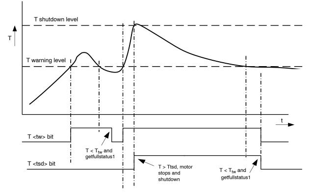
Figure 15. Illustration of Thermal Management Situation
