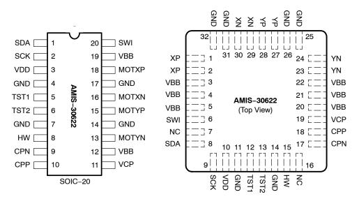
Figure 2. SOIC-20 and NQFP-32 Pin-out
