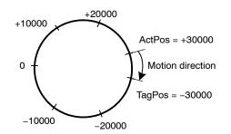
Figure 9. Motion Direction is Function of Difference between ActPos and TagPos
