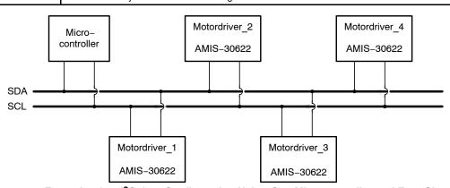
Figure 21. Example of an I<sup>2</sup>C-bus Configuration Using One Microcontroller and Four Slaves
