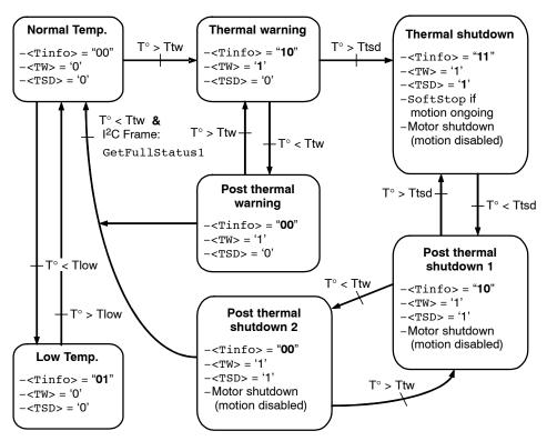
Figure 14. State Diagram Temperature Management
