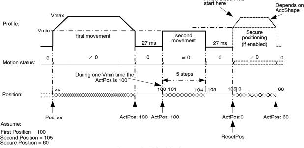
Figure 8. Dual Positioning
