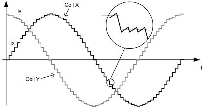
Figure 19. Current Waveforms in Motor Coils X and Y in 1/16<sup>th</sup> Micro-Step Mode
