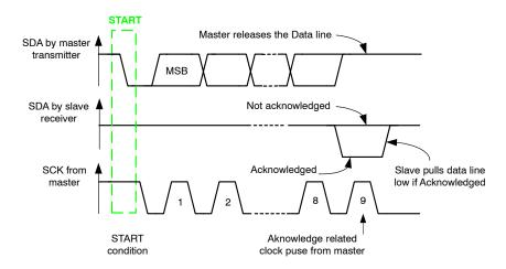
Figure 26. Acknowledge on the I<sup>2</sup>C-bus
