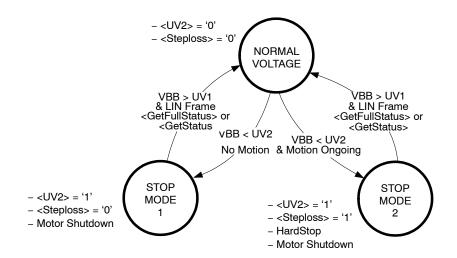
Figure 16. State Diagram Battery Voltage Management
