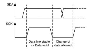
Figure 23. Bit Transfer on the I<sup>2</sup>C-bus
