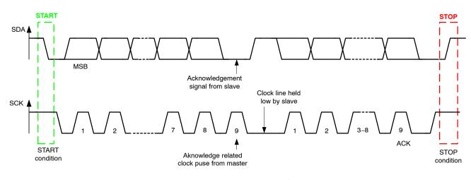
Figure 25. Data Transfer on the I<sup>2</sup>C-bus
