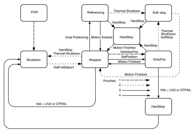
Figure 17. Simplified State Diagram
