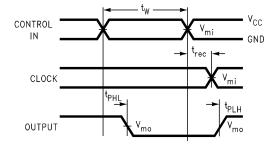
Propagation Delay. Pulse Width and trec Waveforms
