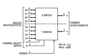
Figure 4. MC74HC4852A Logic Diagram Double-Pole, 4-Position Plus Common Off
