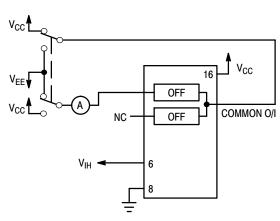
Figure 14. Maximum Off Channel Leakage Current, Any One Channel, Test Set-Up
