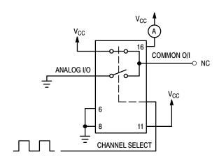
Figure 23. Power Dissipation Capacitance, Test Set-Up
