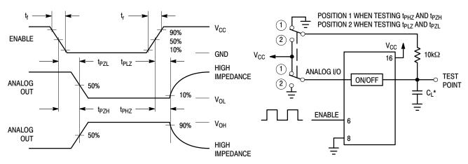
Figure 21. Propagation Delays, Enable to Analog Out
