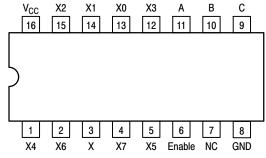
Figure 2. MC74HC4851A 16-Lead Pinout (Top View)
