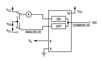
Figure 16. Maximum On Channel Leakage Current, Channel to Channel, Test Set-Up
