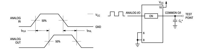
Figure 19. Propagation Delays, Analog In to Analog Out
