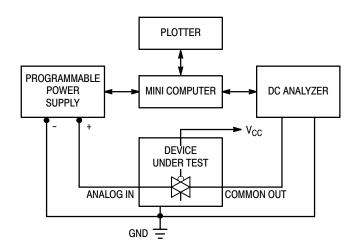
Figure 13. On Resistance Test Set-Up
