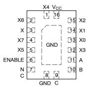
Figure 3. MC74HC4851A QFN Pinout
