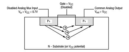
Figure 24. Diagram of Bipolar Coupling Mechanism
