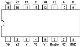
Figure 5. MC74HC4852A 16-Lead Pinout (Top View)
