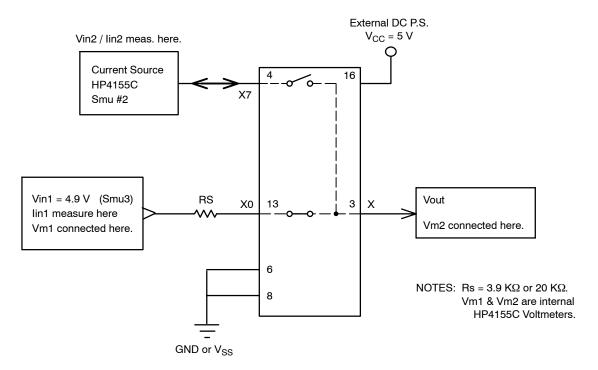
Figure 10. Injection Current Coupling Specification
