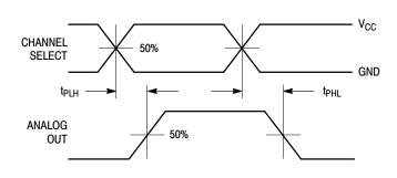
Figure 17. Propagation Delays, Channel Select to Analog Out
