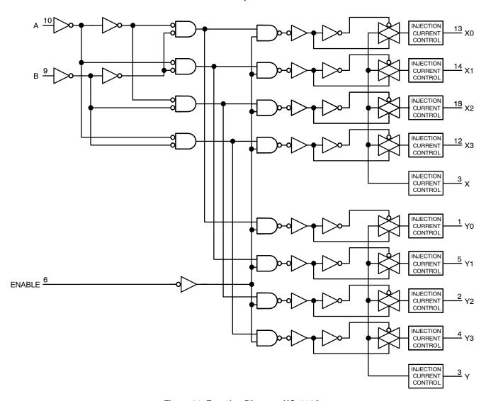
Figure 26. Function Diagram, HC4852A
