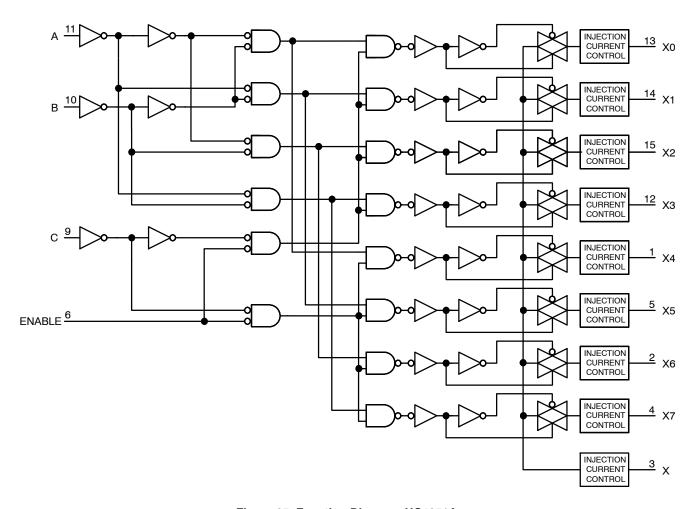
Figure 25. Function Diagram, HC4851A
