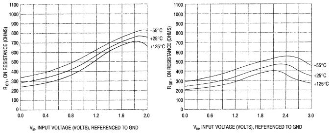
Figure 6. Typical On Resistance V<sub>CC</sub> = 2V
