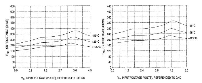
Figure 8. Typical On Resistance  $V_{CC} = 4.5V$
