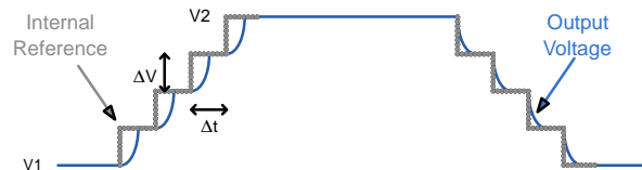
Figure 44. DVS in Forced PPWM Mode Diagram
