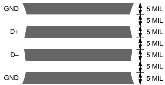
Figure 22. Typical Arrangement of Signal Tracks
