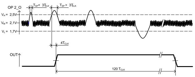
Figure 6. Timing Diagram for Single–Pulse Mode Detection
