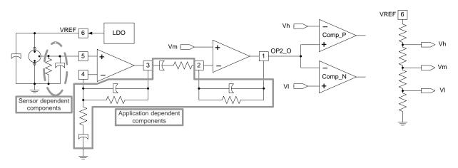
Figure 5. Figure Showing Simplified Block Diagram of Analog Conditioning Stages
