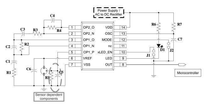
Figure 8. Typical Application Diagram Using NCS36000
