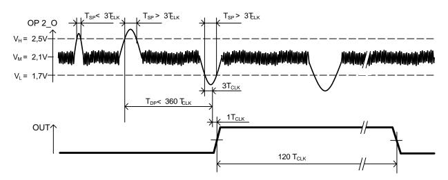
Figure 7. Timing Diagram for Dual-Pulse Mode Detection
