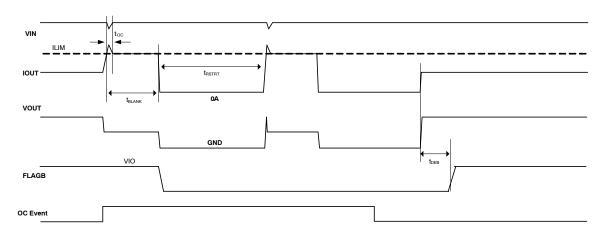
Figure 6. Current Limit Operation (OC\_MODE = HIGH & FLAGB is pulled up with an external VIO)
