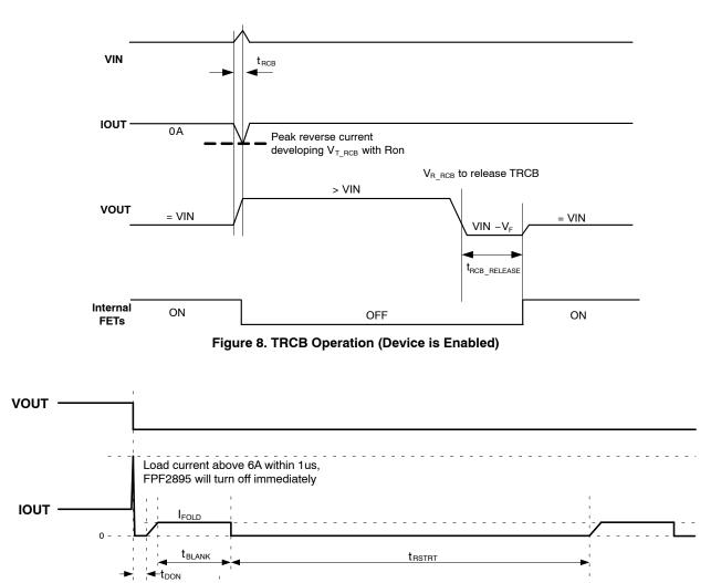
Figure 9. VOUT Hard Short to GND (OC\_MODE = HIGH & FLAGB is pulled up with an external VIO)
