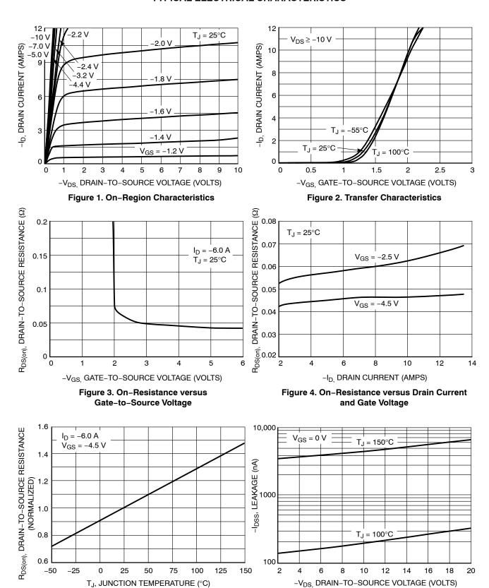
Figure 5. On-Resistance Variation with **Temperature**
