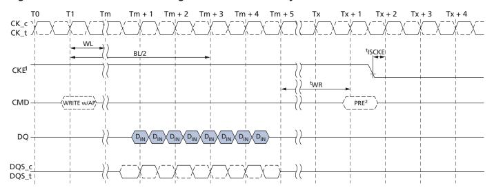
1. CKE can be registered LOW at [WL + 1 + BL/2 + RU(tWR/tCK) + 1] clock cycles after the WRITE command is registered.
