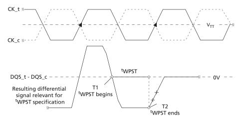
Figure 29: Burst WRITE Followed by Burst READ
