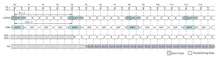
Note: 1. The seamless burst WRITE operation is supported by enabling a WRITE command every four clocks for BL = 8 operation. This operation is supported for any activated bank.
