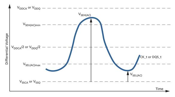
**Note:** While CA and DQ signal requirements are referenced to  $V_{REF}$ , the single-ended components of differential signals also have a requirement with respect to  $V_{DDQ}/2$  for DQS, and  $V_{DDCA}/2$  for CK.
