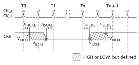
Notes: 1. After CKE is registered LOW, the CKE signal level is maintained below V<sub>ILCKE</sub> for <sup>t</sup>CKE specification (LOW pulse width).
