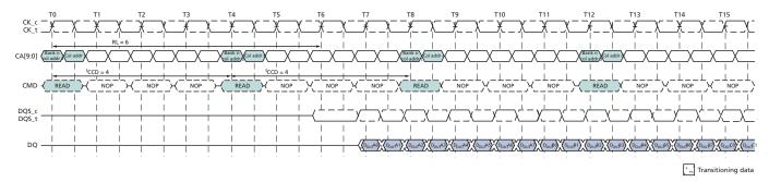
The seamless burst READ operation is supported by enabling a READ command at every fourth clock cycle for BL = 8 operation. This operation is supported as long as the banks are activated, whether the accesses read the same or different banks.
