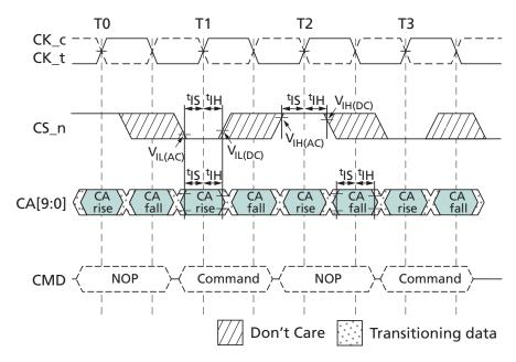
Note: 1. Setup and hold conditions also apply to the CKE pin. For timing diagrams related to the CKE pin, see the Power-Down section.
