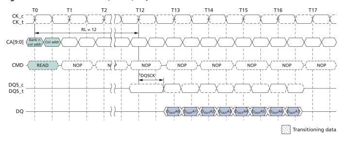
Figure 20: Burst READ Followed by Burst WRITE - RL = 12, WL = 6, BL = 8
