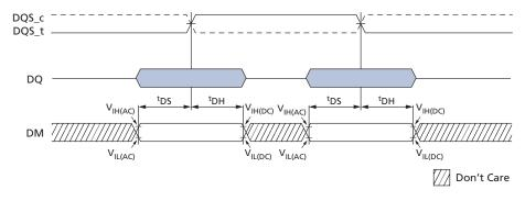
Figure 32: Write Data Mask - Second Data Bit Masked
