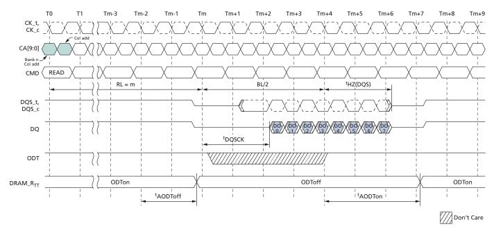
Notes: 1. The automatic R<sub>TT</sub> turn-off delay, <sup>t</sup>AODToff, is referenced from the rising edge of RL - 2 clock at T<sub>m-2</sub>.
