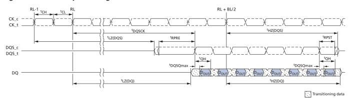
Note: 1. <sup>t</sup>DQSCK can span multiple clock periods.
