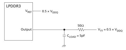
Note: 1. All output timing parameter values (<sup>t</sup>DQSCK, <sup>t</sup>DQSQ, <sup>t</sup>HZ, <sup>t</sup>RPRE, etc.) are reported with respect to this reference load. This reference load is also used to report slew rate.
