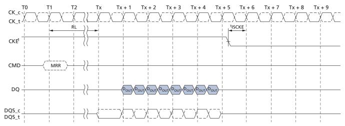
Note: 1. CKE can be registered LOW at [RL + RU(<sup>t</sup>DQSCK/<sup>t</sup>CK)+ BL/2 + 1] clock cycles after the clock on which the MRR command is registered.
