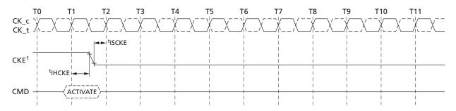
Note: 1. CKE can go LOW at <sup>t</sup>IHCKE after the clock on which the ACTIVATE command is registered.
