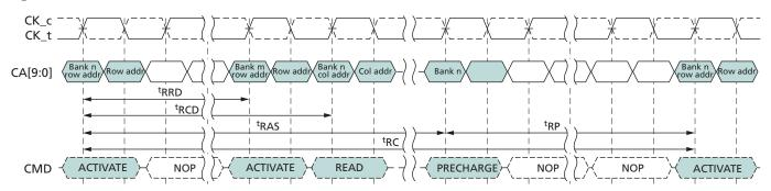
Note: 1. A PRECHARGE ALL command uses <sup>t</sup>RPab timing, and a single-bank PRECHARGE command uses <sup>t</sup>RPpb timing. In this figure, <sup>t</sup>RP denotes either an all-bank PRECHARGE or a single-bank PRECHARGE.
