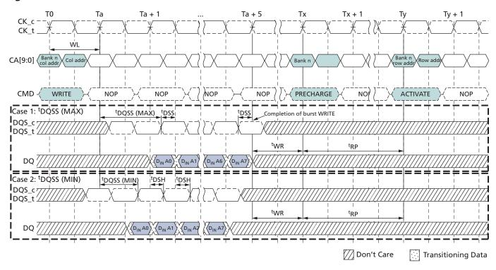
Figure 27: Method for Calculating <sup>t</sup>WPRE Transitions and Endpoints
