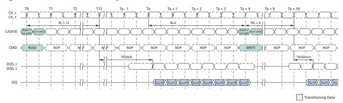
The minimum time from the burst READ command to the burst WRITE command is defined by the read latency (RL) and the burst length (BL). Minimum READ-to-WRITE latency is RL + RU( $^t$ DQSCK(MAX)/ $^t$ CK) + BL/2 + 1 - WL clock cycles.
