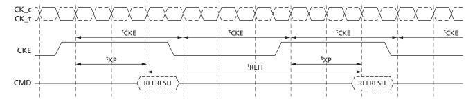
Note: 1. The pattern shown can repeat over an extended period of time. With this pattern, all AC and DC timing and voltage specifications with temperature and voltage drift are ensured.
