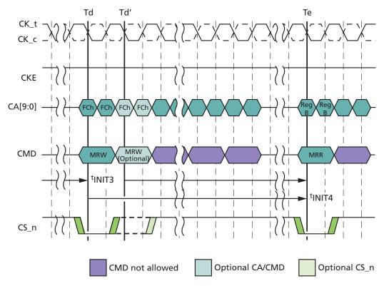
Note: 1. Optional MRW RESET command and optional CS\_n assertion are allowed. When the optional MRW RESET command is used, <sup>t</sup>INIT4 starts at Td'.
