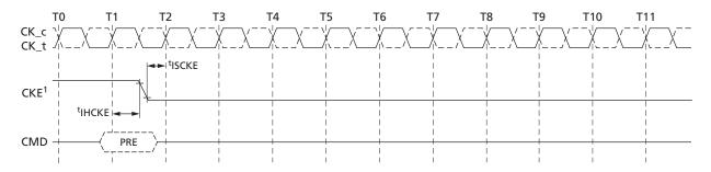
Note: 1. CKE can go LOW <sup>t</sup>IHCKE after the clock on which the PRECHARGE command is registered.
