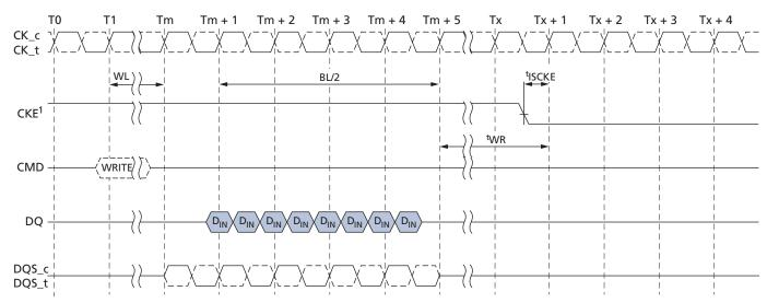
Note: 1. CKE can be registered LOW at [WL + 1 + BL/2 + RU(<sup>t</sup>WR/<sup>t</sup>CK)] clock cycles after the clock on which the WRITE command is registered.
