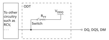
The switch is enabled by the internal ODT control logic, which uses the external ODT pin and other control information. The value of  $R_{TT}$  (ODT termination resistance value) is determined by the settings of several mode register bits. The ODT pin will be ignored if MR11 is programmed to disable ODT in self refresh, in deep power-down, in CKE power-down (mode register option), and during READ operations.
