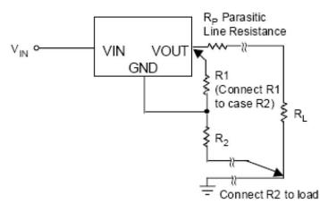
Figure 5. Best Load Regulation Using Adjustable Output Regulator
