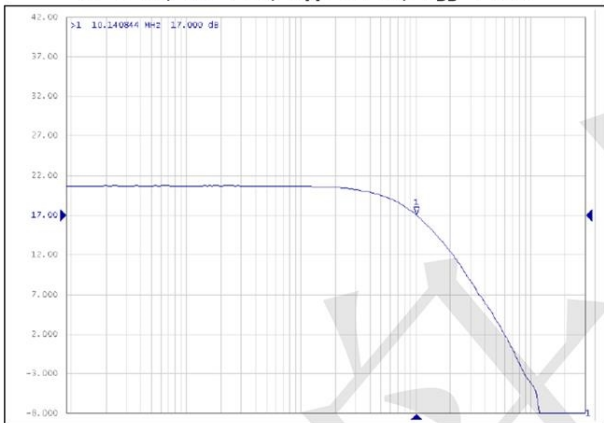
G=+10; RF=2K; V pp =0.2V; V DD =2.5V
