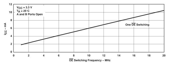
Figure 2. Typical  $I_{CC}$  vs  $\overline{OE}$  Switching Frequency
