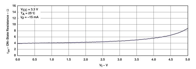
Figure 1. Typical  $r_{on}$  vs  $V_{I}$
