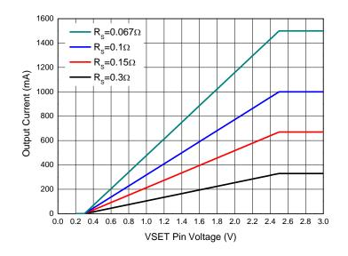
Figure 1. Analog Dimming Curve
