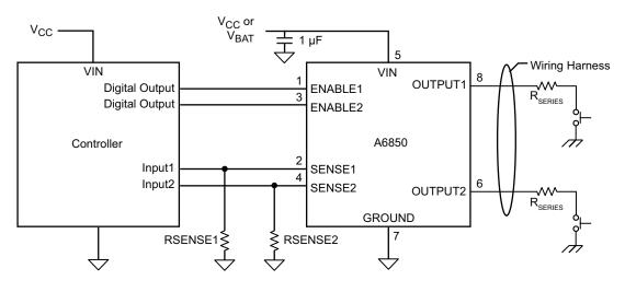
Figure 6. Typical Application with Mechanical Switches
