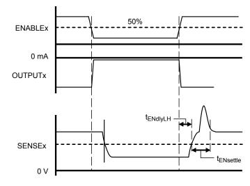
Figure 4. Overshoot resulting from additional capacitance.
