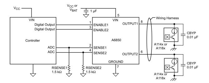
Figure 5. Typical Application with 2-Wire Hall Effect ICs
