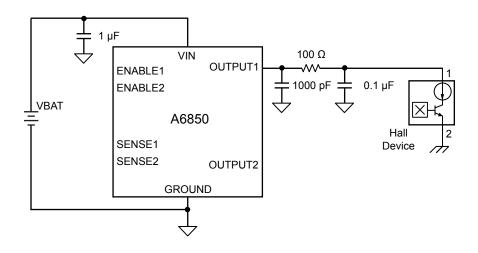
Figure 9. Decoupling and filtering suggestions
