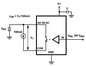
FIGURE 5. ron TEST CIRCUIT
