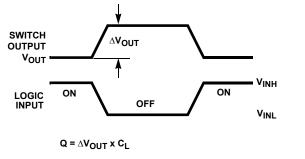
FIGURE 1. SWITCHING TIMES
