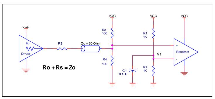
Figure 4. Recommended Schematic for Wiring a Differential Input to Accept Single-ended Levels
