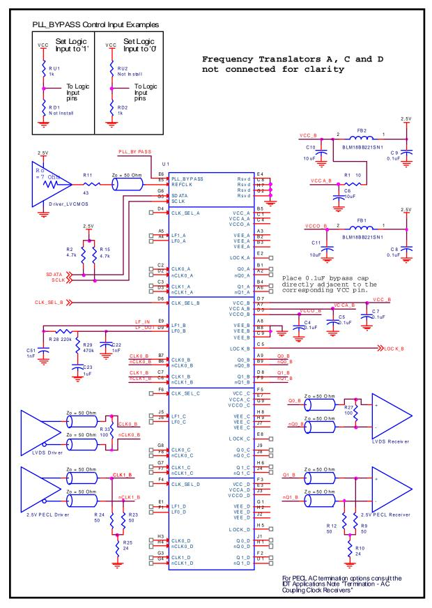
Figure 8. 8T49N488 Schematic Example
