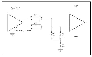
Figure 7B. 2.5V LVPECL Driver Termination Example
