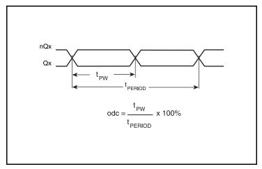
Differential Output Duty Cycle/Output Pulse Width/Period
