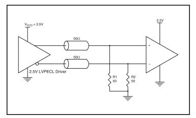
Figure 7C. 2.5V LVPECL Driver Termination Example
