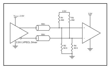
Figure 7A. 2.5V LVPECL Driver Termination Example
