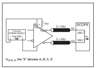
2.5V Core/2.5V LVDS Output Load Test Circuit
