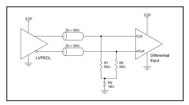
Figure 5B. CLKx/nCLKx Input Driven by a 2.5V LVPECL Driver
