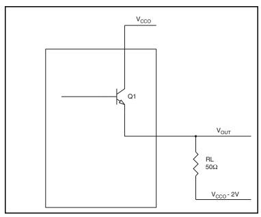
Figure 9. LVPECL Driver Circuit and Termination
