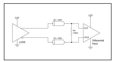
Figure 5D. CLKx/nCLKx Input Driven by a 2.5V LVDS Driver
