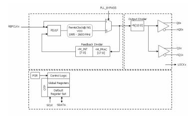
Figure 1. Frequency Synthesizer Mode Block Diagram
