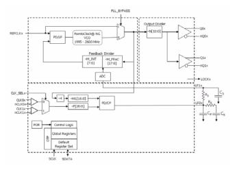
Figure 3. Low Bandwidth Frequency Translator Mode Block Diagram
