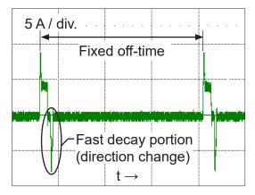
Figure 3. Shorted load (OUTxA  $\rightarrow$  OUTxB) in Mixed decay mode
