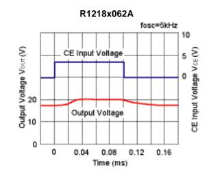
9) PWM Dimming Control (7 LED)  $V_{\text{IN}}$  = 3.6 V, R1 = 10  $\Omega$
