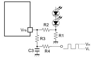
Dimming control by filtered PWM signal
