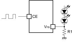
Dimming control by CE pin input
