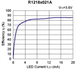
2) Efficiency vs. LED Current (3 LED) L: LQH32CN220 (Ta = 25°C)
