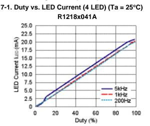
7) PWM Dimming Control (4 LED)  $V_{IN}$  = 3.6 V, R1 = 10  $\Omega$
