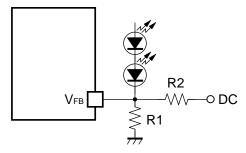
Dimming control by DC voltage
