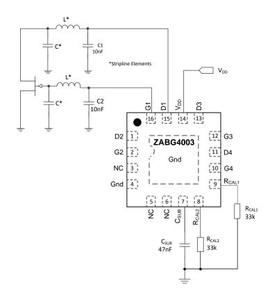
The Gnd flag on the underside ZABG4003 must be connected to ground or left open circuit.
