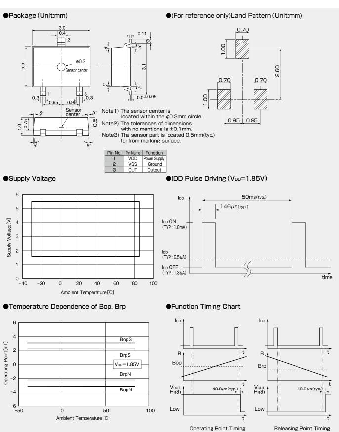
This Hall effect IC's output is held as internal data just before the internal circuit **42** turns OFF (I<sub>DD</sub> OFF). And after 48.8  $\mu$ s, the output changes.
