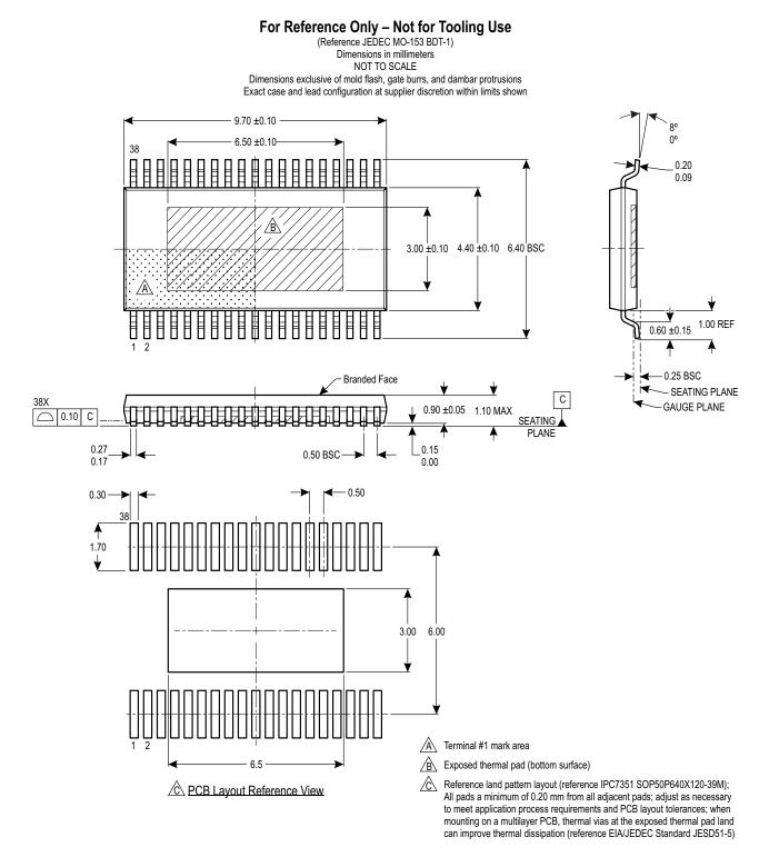
Figure 10: Package LV, 38-Pin eTSSOP
