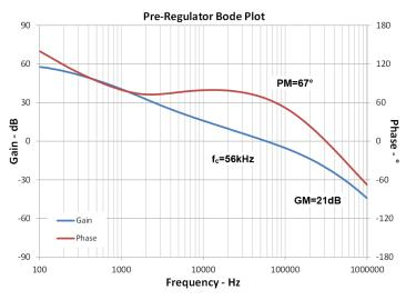
Figure 9: Bode Plot for Pre-Regulator  $R_Z$  = 18.2 kΩ,  $C_Z$  = 3.3 nF,  $C_P$  = 47 pF  $L_O$  = 4.7 µH,  $C_O$  = 3 × 10 µF (16V/X7R/1206) MLCC
