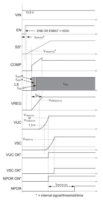
Figure 2: Startup Timing Diagram
