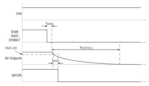
All outputs start to decay  $t_{d(\mathrm{EN})}$  seconds after ENB and ENBAT are low.
