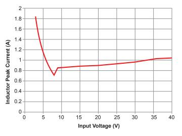
Figure 8: Typical Peak Inductor Current versus Input Voltage for 0.8 A Output Current and 10 µH Inductor
