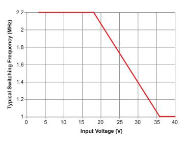
Figure 7: Typical Switching Frequency versus Input Voltage
