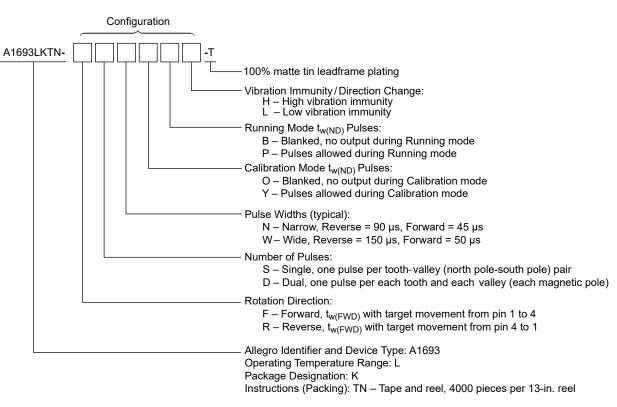
All variants: Target configuration is ring magnet, device should be back-biased for ferromagnetic target operation.
