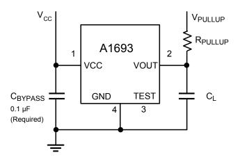
**Figure 10: Typical Application Circuit**
