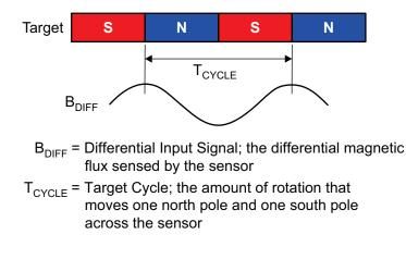
Figure 1: Definition of T<sub>CYCLE</sub>
