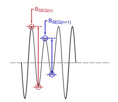
Figure 3: Definition of Differential Signal Variation
