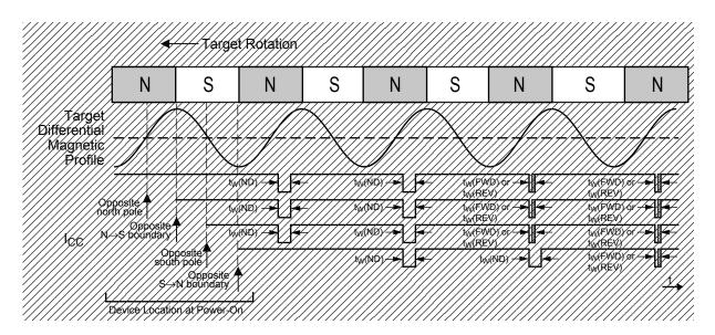
Figure 8: Start-up position effect on first device output switching (Option Y shown: pulse-in-calibration)
