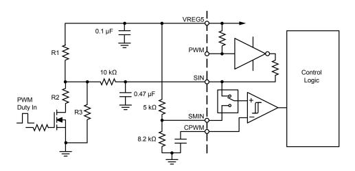
PWM control using External PWM input
