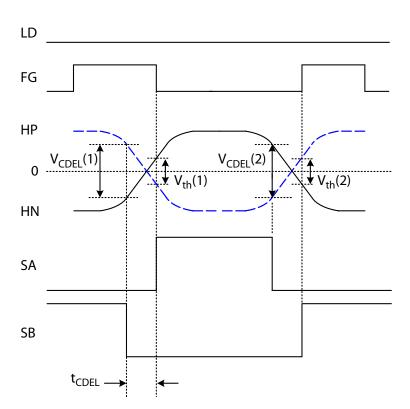
$$V_{th}(1) = V_{HP} - V_{HN} = 10 \text{ mV (Typical)}$$
