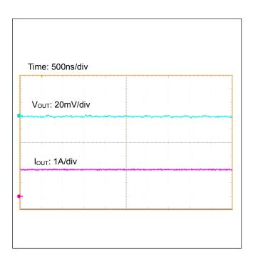
Figure 60. Output Ripple Voltage (IOUT=2A)
