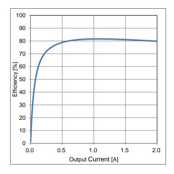
Figure 52. Efficiency vs Output Current
