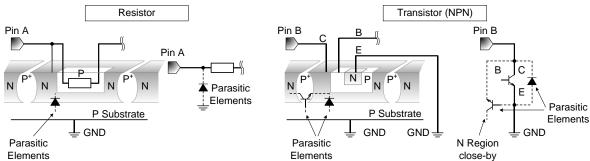
Figure 74. Example of monolithic IC structure
