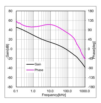
Figure 53. Frequency Characteristics (I<sub>OUT</sub>=2A)
