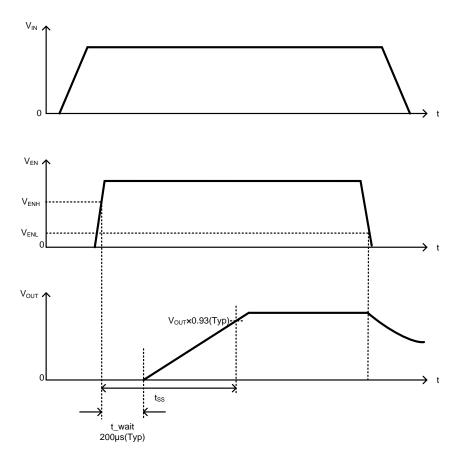
Figure 24. Enable ON/OFF Timing Chart
