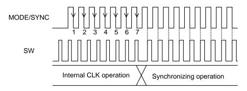
Figure 26. External Synchronization Function Timing Chart
