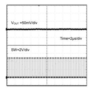
Figure 30. SW Waveform (Forced PWM Control) (V<sub>IN</sub>=5.0V, V<sub>OUT</sub>=1.8V, I<sub>OUT</sub>=1A)
