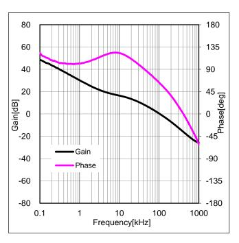
Figure 43. Frequency Characteristics (I<sub>OUT</sub>=2A)
