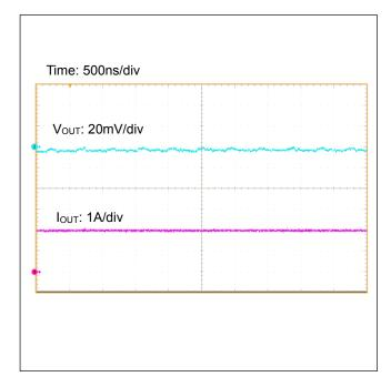
Figure 55. Output Ripple Voltage (I<sub>OUT</sub>=2A)
