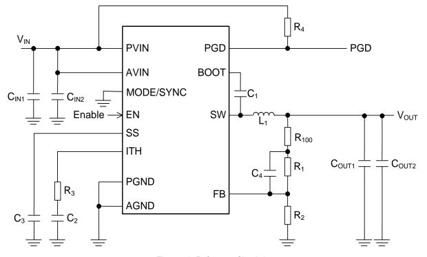
Figure 51. Reference Circuit 3
