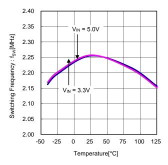
Figure 6. Switching Frequency vs Temperature
