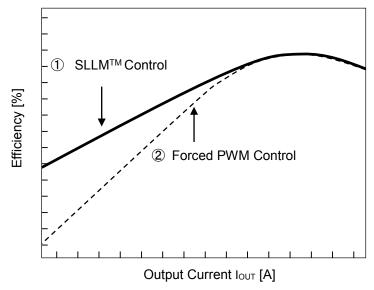
Figure 28. Efficiency (SLLM<sup>TM</sup> Control and Forced PWM Control)
