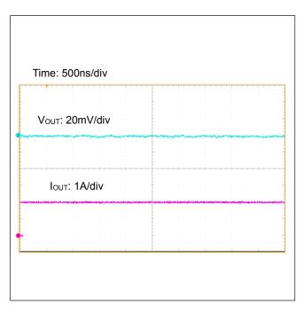
Figure 45. Output Ripple Voltage  $(I_{OUT}=2A)$
