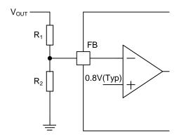
Figure 35. Feedback Resistor Circuit
