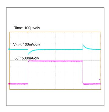
Figure 59. Load Transient Response (I<sub>OUT</sub> = 0A↔2A)
