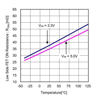
Figure 15. Low Side FET ON Resistance vs Temperature
