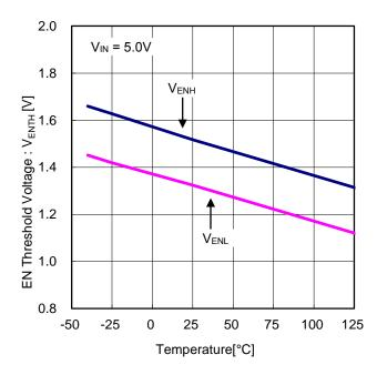
Figure 19. EN Threshold Voltage vs Temperature
