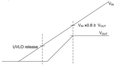
Figure 40. Input Voltage Startup Time
