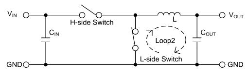
Figure 71-b. Current Path when H-side Switch = OFF, L-side Switch = ON
