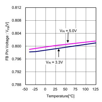
Figure 7. FB Pin Voltage vs Temperature
