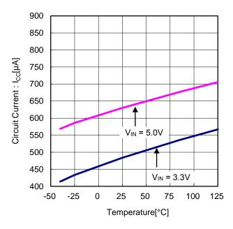
Figure 4. Shutdown Circuit Current vs Temperature
