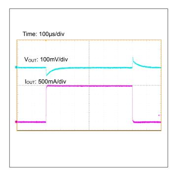
Figure 54. Load Transient Response (I<sub>OUT</sub>=0A↔2A)
