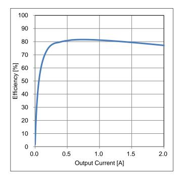
Figure 42. Efficiency vs Output Current
