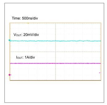
Figure 49. Load Transient Response (Iou⊤=0A↔2A)
