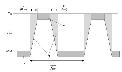
Figure 73. SW Waveform
