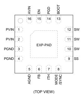
Figure 2. Pin Configuration
