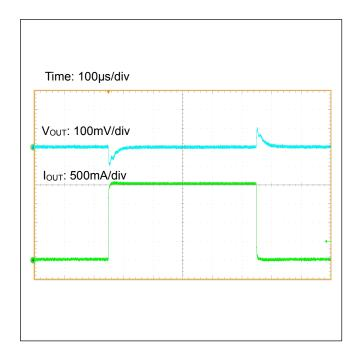
Figure 64. Load Transient Response ( $I_{OUT}=0A \leftrightarrow 2A$ )
