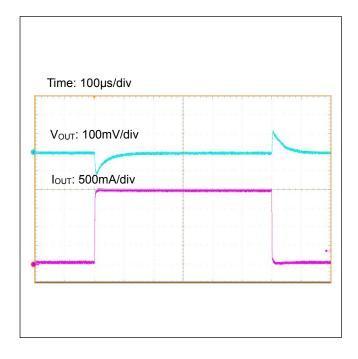
Figure 44. Load Transient Response  $(I_{OUT}=0A\leftrightarrow 2A)$
