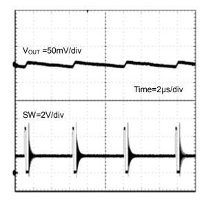
Figure 29. SW Waveform (SLLM<sup>TM</sup> Control) (V<sub>IN</sub>=5.0V, V<sub>OUT</sub>=1.8V, IOUT=50mA)
