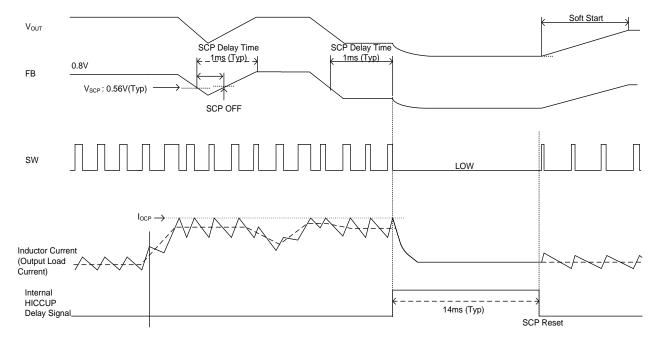
Figure 31. Short Circuit Protection (SCP) Timing Chart
