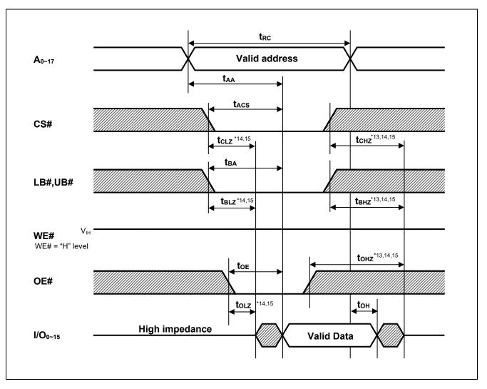
Note 13. t<sub>CHZ</sub>, t<sub>BHZ</sub> and t<sub>OHZ</sub> are defined as the time when the I/O pins enter a high-impedance state and are not referred to the I/O levels.
