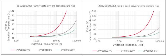
\*Assumptions for above curves:  $T_a = 25$  °C,  $V_{BUS} = 400$  V,  $V_{CC} = 12$  V,  $R_{gon} = 10$   $\Omega$ ,  $R_{goff} = 5\Omega$
