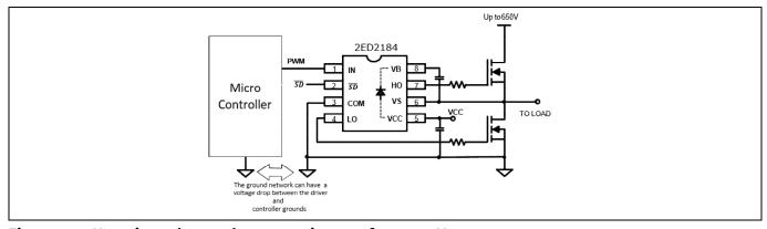
Figure 18 Negative voltage tolerance on inputs of upto -5 V
