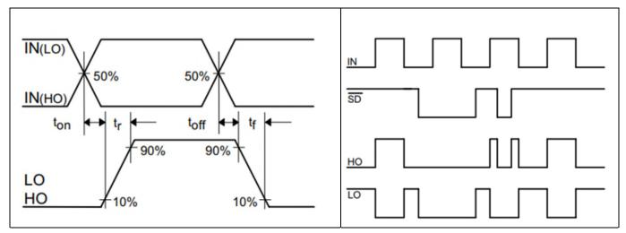
Figure 6 Switching timing diagram
