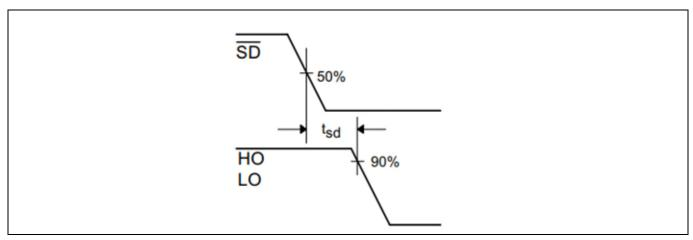
Figure 14 Shutdown waveform definitions
