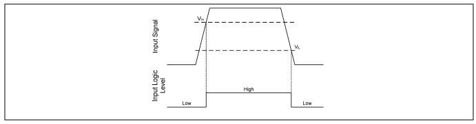
Figure 12 IN input thresholds
