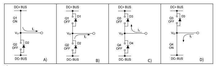
Figure 20 A) Q1 conducting B) D2 conducting C) D3 conduct
