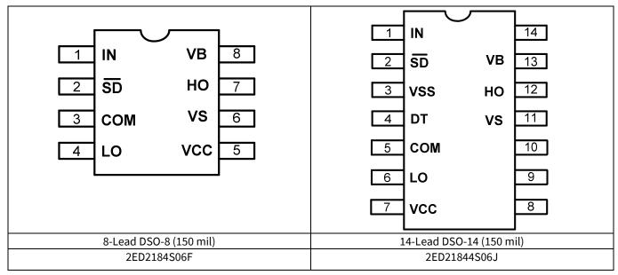
Figure 3 2ED2184(4)S06F(J) pin assignments (top view)
