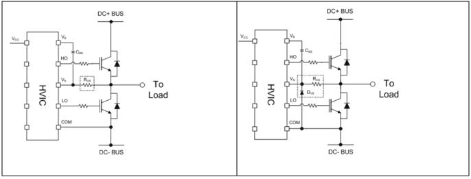
Figure 26 Resistor between the VS pin and the switch node
