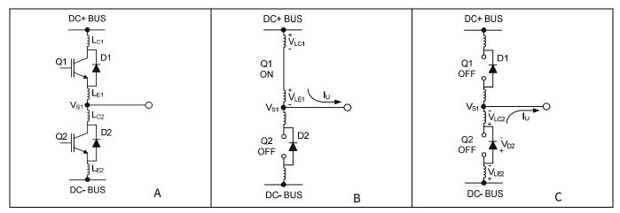
Figure 21 Figure A shows the Parasitic Elements. Figure B shows the generation of  $V_s$  positive. Figure C shows the generation of  $V_s$  negative
