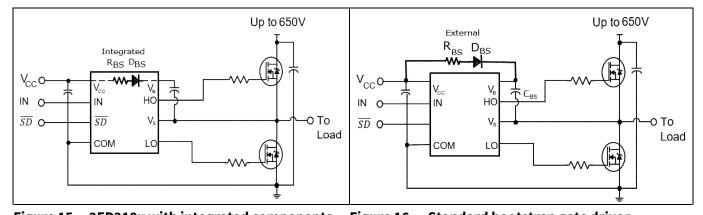
Figure 15 2ED218x with integrated components Figure 16 Standard bootstrap gate driver
