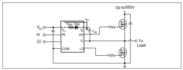
Figure 17 Half bridge bootstrap circuit in 2ED218x
