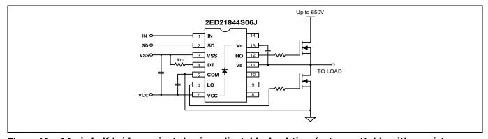
Figure 10 14-pin half-bridge variants having adjustable dead-time feature settable with a resistor
