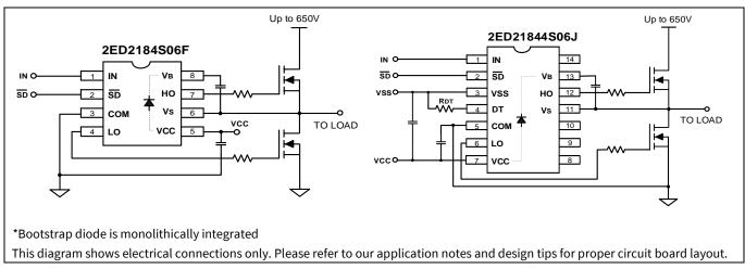
Figure 1 Typical application block diagram
