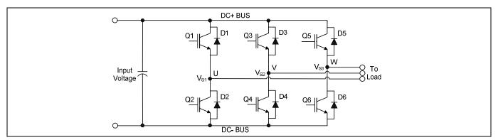
Figure 19 Three phase inverter
