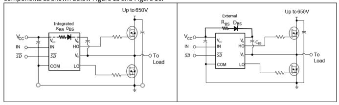
Figure 15 2ED210x with integrated components
