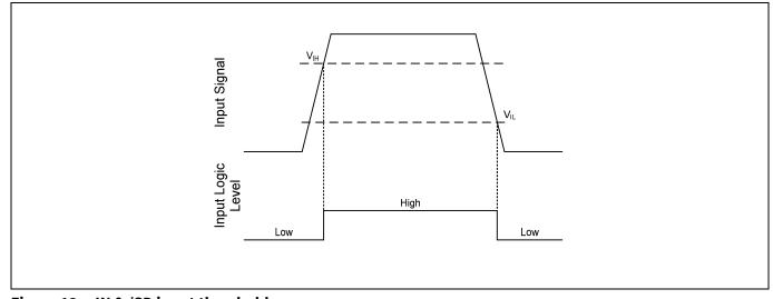
Figure 13 IN & /SD input thresholds
