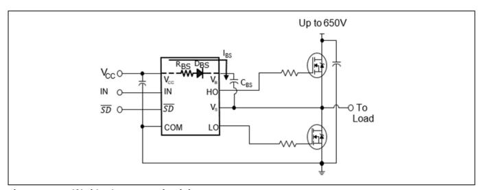
Figure 17 Half bridge bootstrap circuit in 2ED210x
