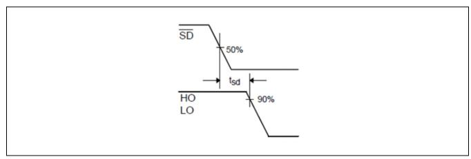
Figure 12 Shutdown waveform definitions
