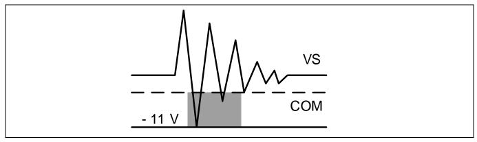
Figure 23 Headroom for HV level shifter data transmission
