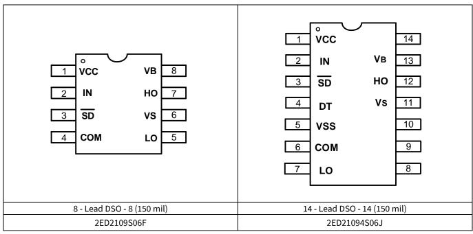
Figure 3 2ED2109 (4) S06 F(J) pin assignments (top view)
