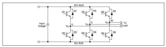
Figure 19 Three phase inverter
