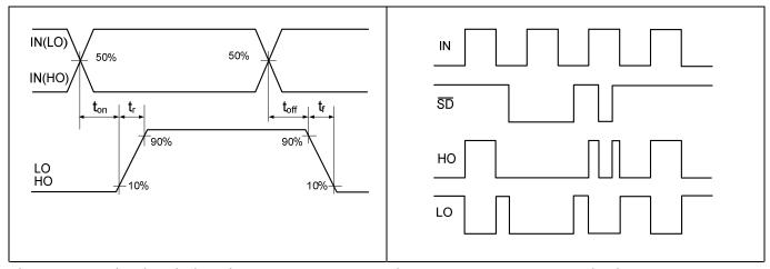
Figure 6 Switching timing diagram
