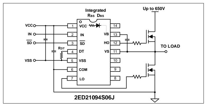
Figure 9 14-pin half-bridge variants having adjustable dead-time feature settable with a resistor
