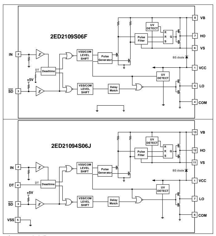
Figure 2 Block diagrams
