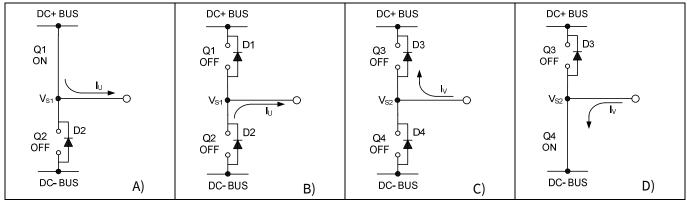
Figure 20 A) Q1 conducting
