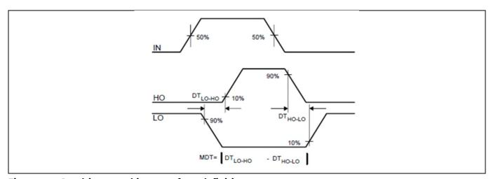
Figure 8 Deadtime matching waveform definition
