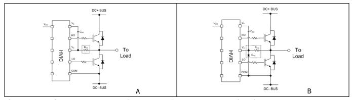
Figure 26 Resistor between the VS pin and the switch node and clamping diode between COM and VS
