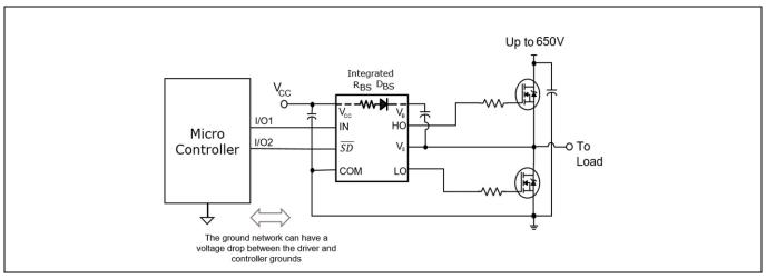
Figure 18 Negative voltage tolerance on inputs of upto -5 V
