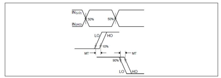
Figure 11 Deadtime matching waveform definition
