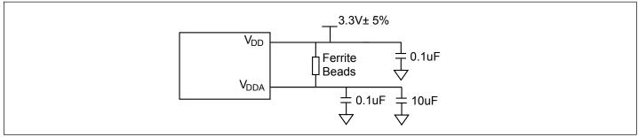
Figure 3. Power Supply Filter
