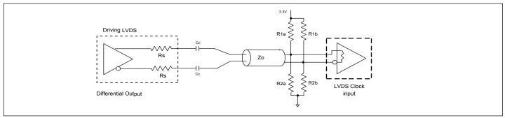
Figure 2. Differential Output Driving LVDS
