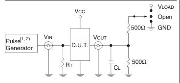
Test Circuits for All Outputs
