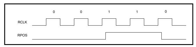
FIGURE 15. DUAL RAIL MODE WITH A FIXED REPEATING "0011" PATTERN
