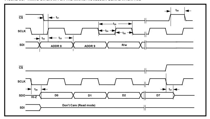
Table 14: Microprocessor Serial Interface Timings (  $T_A = 25^{0}$ C,  $V_{DD} = 3.3V \pm 5\%$  and load = 10pF)
