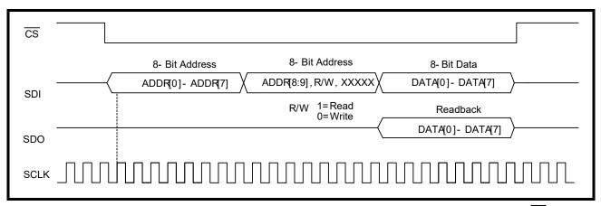
**Note:** For applications without a free running SCLK, a minimum of 1 SCLK pulse must be applied when CS is "High", befrore pulling  $\overline{\text{CS}}$  "Low".
