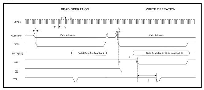
TABLE 21: MOTOROLA MPC86X MICROPROCESSOR INTERFACE TIMING SPECIFICATIONS
