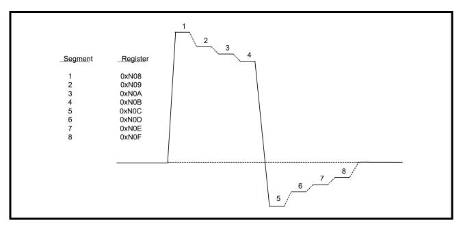
**Note:** By default, the arbitrary segments are programmed to 0x00h. The transmitter outputs will result in an all zero pattern to the line interface.
