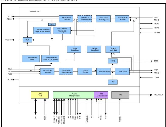
FIGURE 1. BLOCK DIAGRAM OF THE XRT83VSH316
