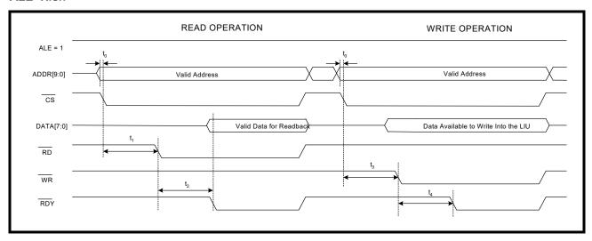
TABLE 20: INTEL MICROPROCESSOR INTERFACE TIMING SPECIFICATIONS
