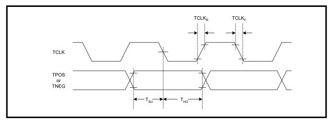
FIGURE 19. TRANSMIT DATA SAMPLED ON RISING EDGE OF TCLK
