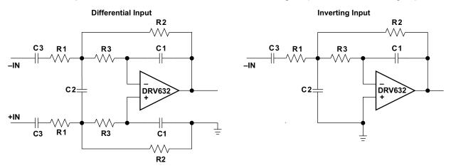
Figure 8. Second-Order Active Low-Pass Filter
