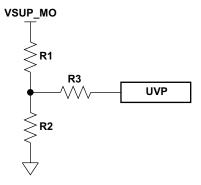
Figure 7. UVP Resistor Divider
