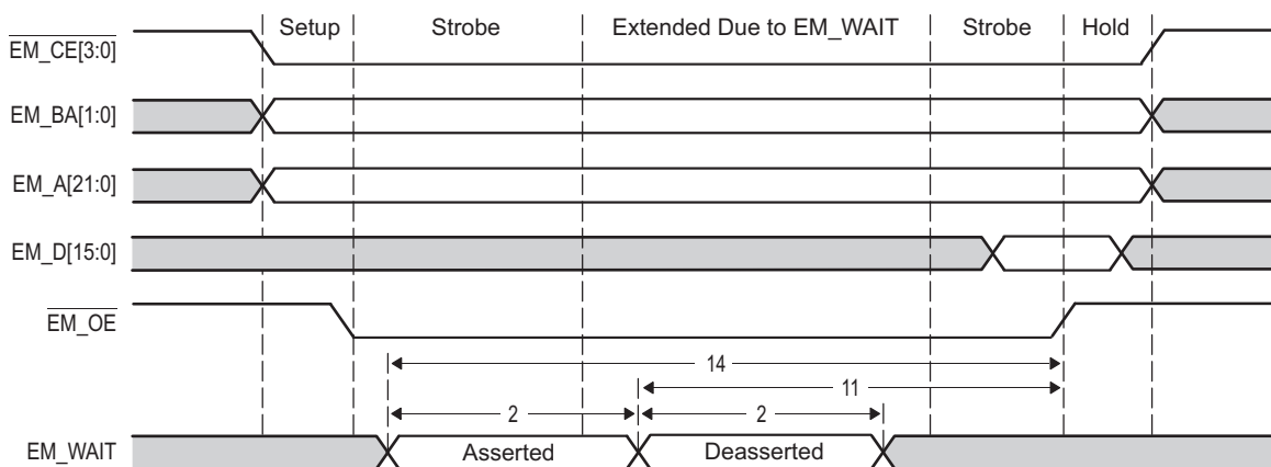
Figure 11-54. EMIF16 EM_WAIT Read Timing Diagram
