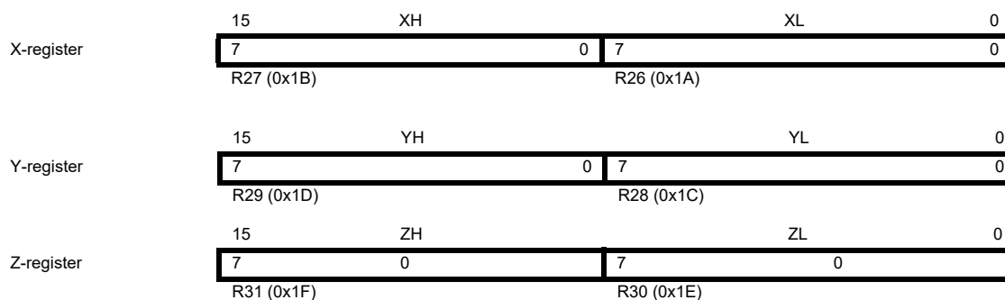
Figure 7-3. The X-, Y-, and Z-registers
