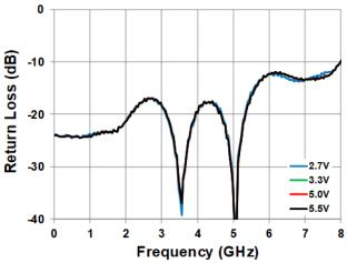
Figure 17. Typical RFX Return Loss vs. Frequency over V<sub>DD</sub> [Selected State]
