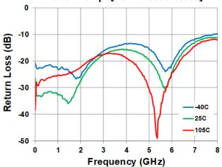
Figure 24. Return Loss (During Switching) vs.
