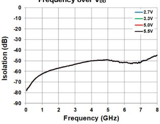
Figure 12. RFX to RFX Isolation vs. Frequency
