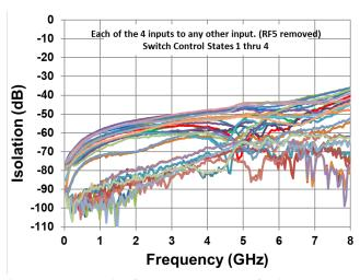
Figure 14. Typical RFX to RFX Isolation vs. Frequency over VDD
