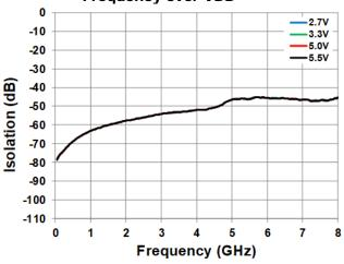
Figure 11. RFX to RFX Isolation vs. Frequency
