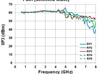
Figure 32. RF2 IIP3 vs. Frequency over Temperature and Voltage
