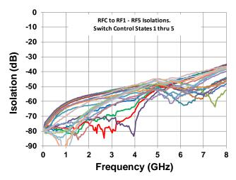
Figure 9. Typical RFC to RFX Isolation vs. Frequency over Temperature
