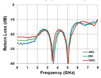
Figure 21. RFX Return Loss vs. Frequency over Switch Path [Terminated State]
