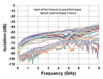
Figure 13. Typical RFX to RFX Isolation vs. Frequency over Temperature
