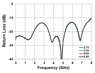
Figure 19. Typical RFC Return Loss vs. Freq. over Temp. [Selected State]
