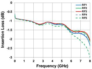
Figure 6. Insertion Loss vs. Frequency over Voltage
