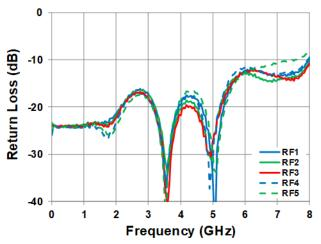
Figure 20. Typical RFC Return Loss vs. Freq. over V<sub>DD</sub> [Selected State]
