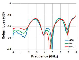
Figure 18. RFC Return Loss vs. Frequency over Switch Path [Selected State]
