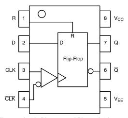
Figure 1. Logic Diagram and Pinout Assignment
