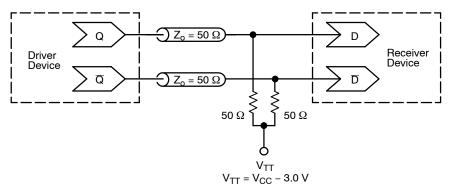
Figure 2. Typical Termination for Output Driver and Device Evaluation (See Application Note <u>AND8020/D</u> – Termination of ECL Logic Devices.)
