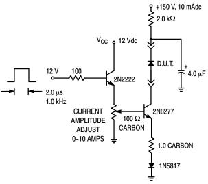
Figure 6. Test Circuit for Repetitive Reverse Current
